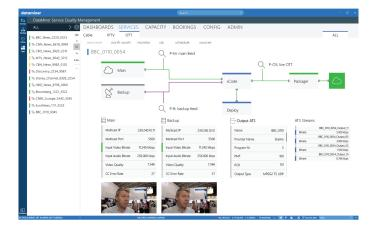
ORION-OTT's integration with DataMiner offers an automated end-to-end solution ensuring Quality of Service (QoS) and Quality of Experience (QoE). The integration provides service assurance for linear and non-linear channels.
